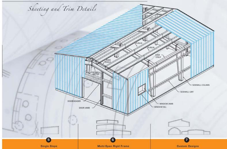
Available in clear and multi-span applications. A Single Slope provides drainage to one side, directing runoff away from building facades, entrances or parking areas. Designed for large buildings, using a minimum of interior columns. Ideal for manufacturing, warehousing, retail space, offices and multiple industrial applications.
